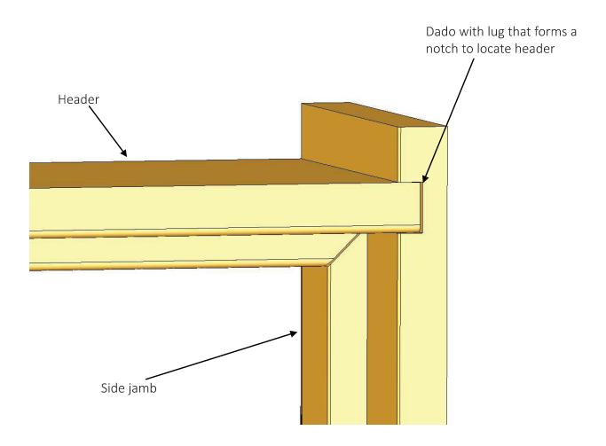
This method is not commonly used due to the fact that the lug has to be cut-off to install the door unit in the opening. The advantage of this method is that it holds the location of the header secure during shipping.
